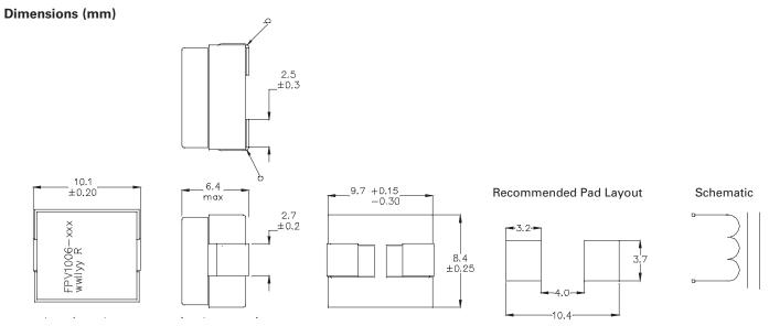
Part marking: FPV1006–xxx, xxx=inductance value in nH, wwllyy= date code, R=revision level Tolerances are ±0.25 unless stated otherwise Soldering surfaces to be coplanar within 0.102 millimeters DCR measured from point "a" to point "b" Do not route traces or vias underneath the inductor.
